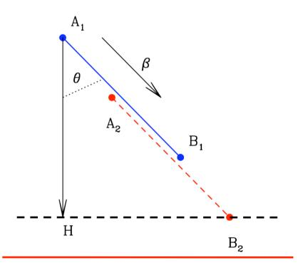
The photon emitted in A1 at  $t=t_i$  after a time  $\Delta t_e$  reaches H. In the meantime, the bar moves from its initial position  $A_1B_1$  to the final one  $A_2B_2$ . The photon emitted in  $B_2$  reaches the detector at the same time of the photon emitted at earlier times in  $A_1$ .
